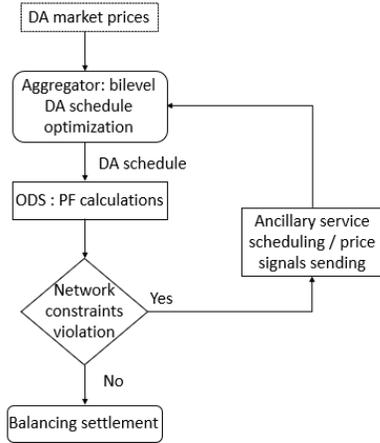
Figure 1 Coordination model between the DSO and the aggregator
