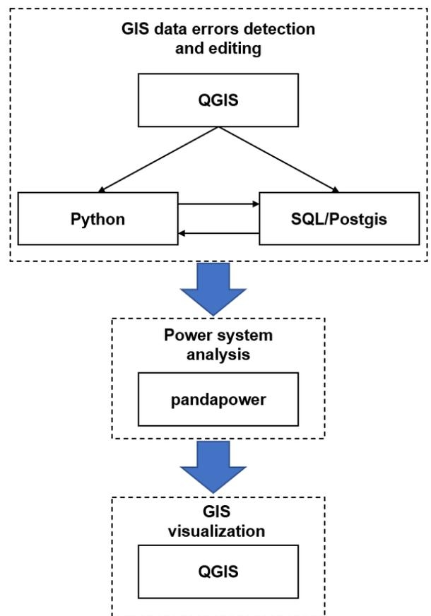
Fig. 1 Flow chart of the integrated tool
